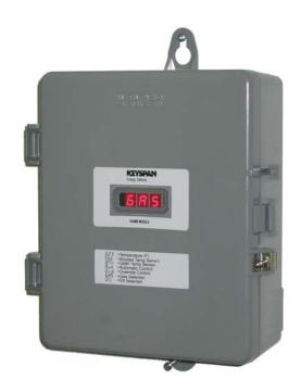
The K322 has the ability to automatically switch the controlled site to an oil or gas fuel source based on the measured site temperature. If enabled, the K322 will switch to oil when the temperature drops below a programmable setpoint and back to gas when the temperature rises above a second setpoint.
